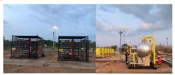
Surface production test at 9 November 2023 results well SED#4 4500 bopd flowing well by 12/64" and 16/64" choke. Well SED#3 pumped by ESP Reda 180 HP results 3800 bopd.
